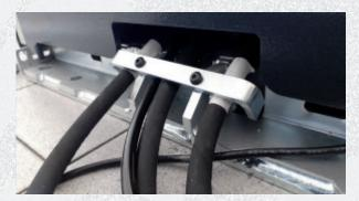
For this purpose, should it become necessary to replace the hydraulic hoses due to premature wear, we recommend the installation of the above support, if not present, in the lift models listed below:
